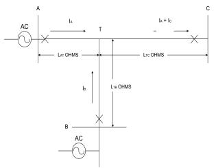
On lines with tee-off transformers connected to them, the tee-off transformers can supply zero sequence current if they are earthed on the line side. This is equivalent to an infeed as indicated and must be taken into account when choosing the Zone 2 setting. Normally the Zone 2 reach will be set so that it does not extend beyond a power transformer, but should a particular application require an extended reach of this nature, then care should be taken to grade the protection accordingly.
