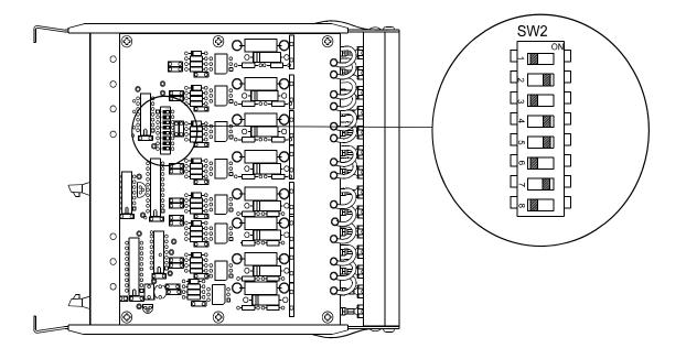
Note: Switch SW2 controls 8 status inputs. As supplied, all switches are in the left hand position and all status inputs are high speed devices.
